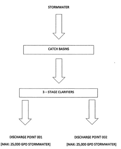
\* TOTAL: MAX 50,000 GPD STORMWATER RUNOFF \*
